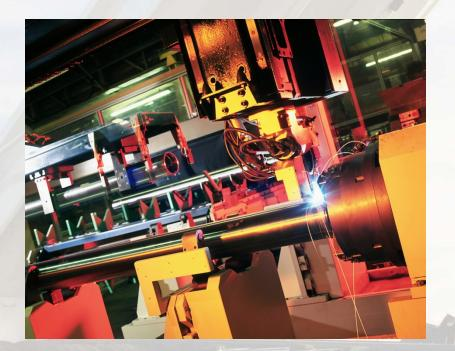
High grade alloy steel, thin wall tubing and laser welding technology for unique high performance cylinder construction
